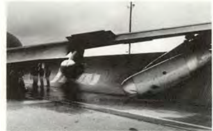
Wandering heavy vs blast fence after loss of nose wheel steering and brakes. A combination of errors resulted in two mis-positioned cockpit switches. Just a little thing. . . .
