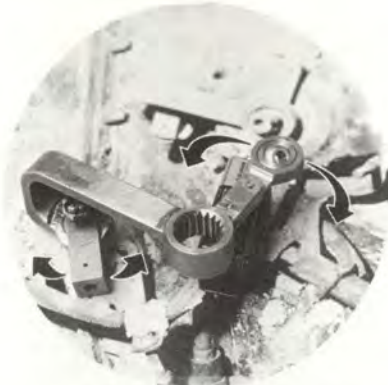
Broken feedback cable due to bending loads imposed by frozen uniball in actuating layer. This resulted in engine failure and a destroyed aircraft.
