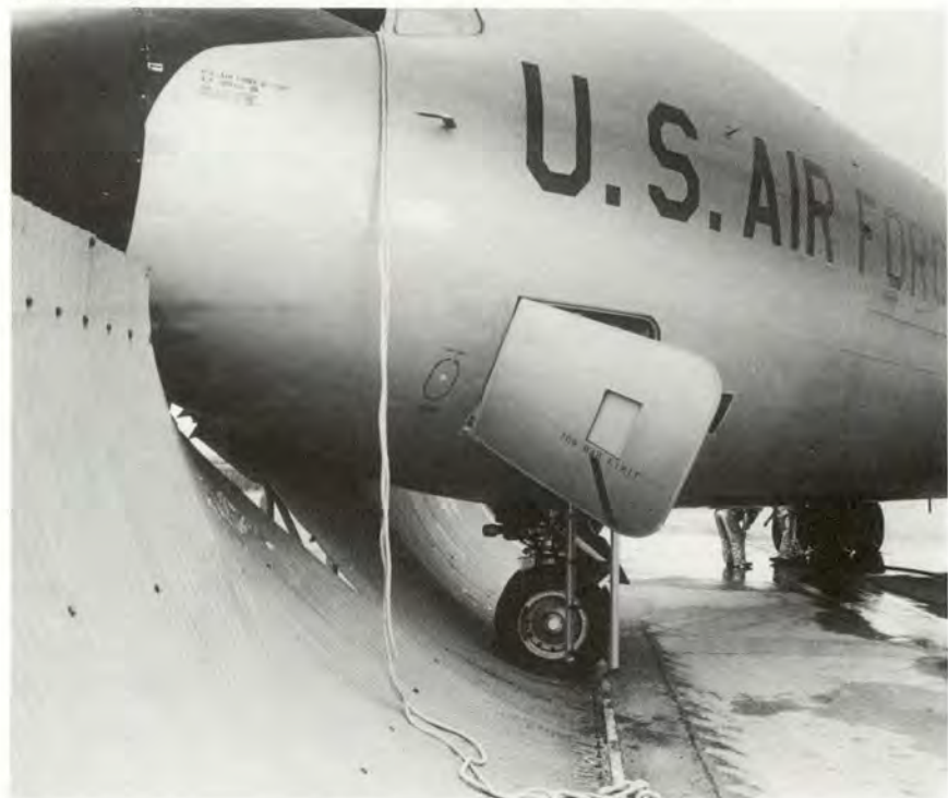
Wandering heavy vs blast fence after loss of nose wheel steering and brakes. A combination of errors resulted in two mis-positioned cockpit switches. Just a little thing. . . .
